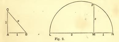
may construct an isosceles right-angled triangle ABC such that AB = AC = 1. Then if BC = x,  $x^2 = 2$ . Or we may determine the length x by means of Euclid's construction (Euc. VI. 13) for a mean proportional to 1 and 2, as indicated in the figure. Our requirements therefore involve the existence of a length measured by a number x, and a point P on  $\Lambda$  such that
