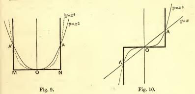
The reader should next consider the curves given by  $y=x^m$ , when *m* is odd. The fundamental difference between the two cases is that whereas when *m* is even  $(-x)^m = x^m$ , so that the curve is symmetrical about OY, when *m* is odd  $(-x)^m = -x^m$ , so that y is negative when x is negative. Fig. 10 shows the curves y = x,  $y = x^3$ , and the form to which  $y = x^m$  approximates for larger odd values of m
