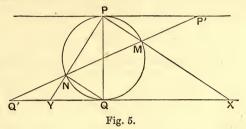
Take PP' = -2a/b and QQ' = -c/2b, having regard to sign\*. Join P'Q', cutting the circle in M and N. Draw PM and PN, cutting QQ' in X and Y. Then QX and QY are the roots of the equation with their proper signs  $\dagger$ .
