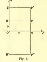
**OAPB.** Imagine the point P marked on the diagram. This marking of the point P may be regarded as showing that the value of y for x = a is b.
